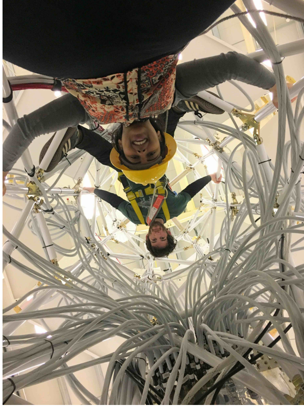
Figure 2.5: Andrew Ludwig and I working on integration and cabling of ANITA-4 at the NASA LDB facility near McMurdo Station, Antarctica. The aluminum beams that form the underlying structure of the payload can be seen here. Light aluminum beams help to abide by weight restrictions. Image credit: Nan Wang.
